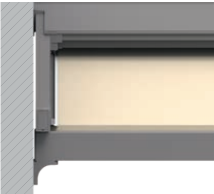
Installation of the guttering laterally on a wall using the guttering angle bracket
